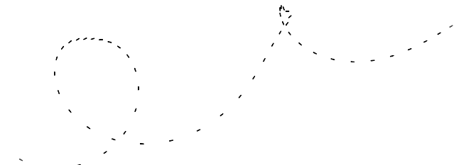
c) Inertial 2-D view of the midspan section, time 25–50 s (showing pitch loops)
